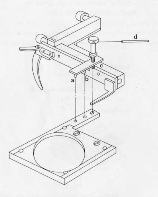
This mechanical stage is specially designed to be used with this field microcope and is quite useful.
