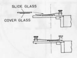
Position ILLUMINATOR BRACKET and secure by KNURLED SCREW in line with the countersunk groove.
