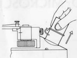
Place (inverted) specimen slide on stage (specimen or cover glass down).
