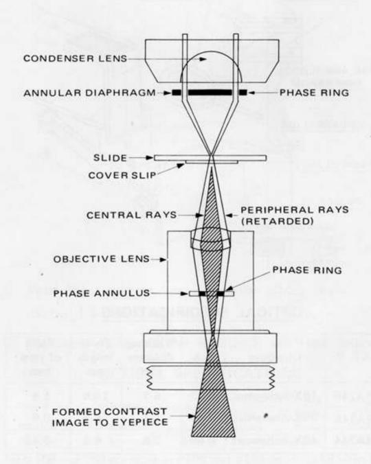
This phase system provides an image of hard-to-see specimens in their natural, living condition, by a method of optical staining.
